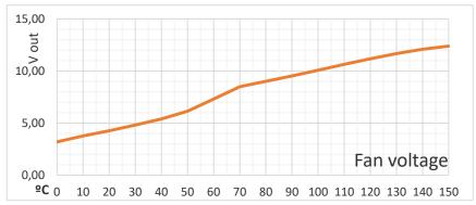
If this voltage reaches 6V, a 12V fan will start by "nature" and speeding up with temperature rising. While using a correct sized fan, it all will stabilize at an acceptable temperature, since the rotating fan is cooling the amp, the voltage drops, the vent turns slower, etc.......
